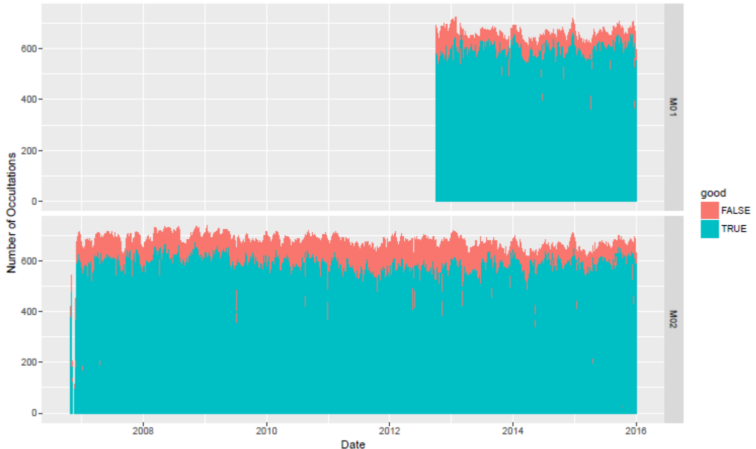
Fig. 2.2: Daily number of “good” (i.e., successfully processed; blue) and “bad” (red) occultations from the GRAS instruments onboard Metop-A (top) and -B (bottom) during the reporting period.
