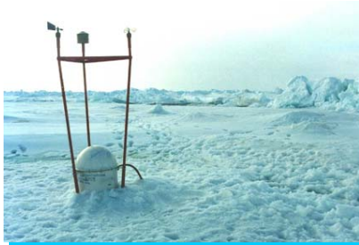
Meteorological ice drifting buoy using for IABP and IPAB
