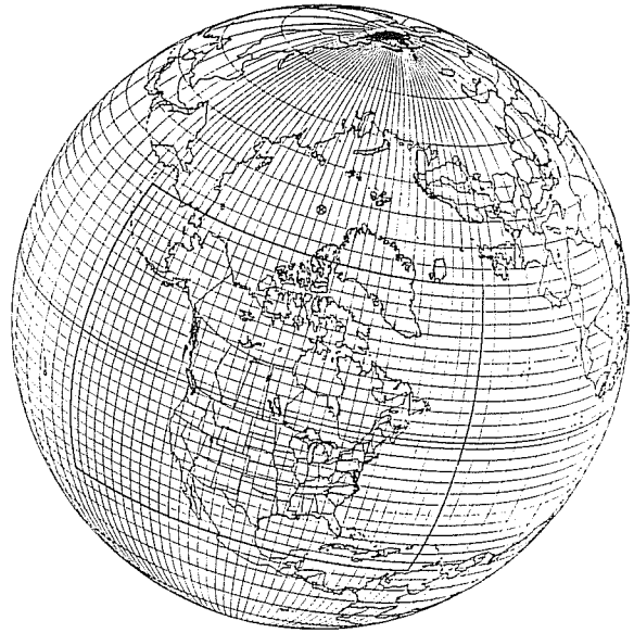
Fig.6(b) A variable-resolution 162 \times 120 mesh having an 81.6^\circ \times 60^\circ window of uniform 0.8^\circ resolution, centered on (103^\circ\text{W}, 51^\circ\text{N}) , and used for Expt B: for clarity only every 3rd point in each direction is plotted.
