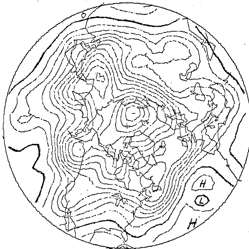
Fig. 2. A suspicious case from 1965-12-23:00. The small low in the middle of the Azores high is absent in the preceding analysis (1965-12-22:12) and in the following analysis (1965-12-23:12). A deeper synoptic study is required in order to decide which one of the analyses is wrong.
