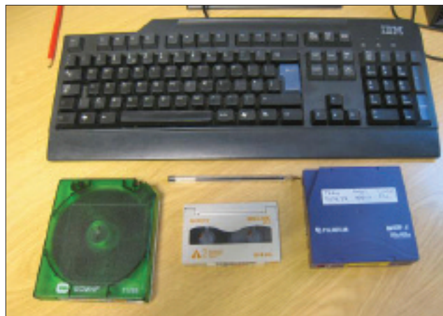
Figure 1 The different cartridges are shown: Magstar on the left, AIT in the middle and LTO-3 on the right.
