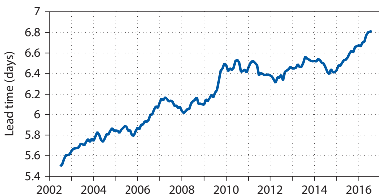
Skill of the HRES as measured by ECMWF's primary deterministic headline score. Results for geopotential at 500 hPa in the northern hemisphere extra-tropics show that the medium-range forecast skill continues to increase due to recent model upgrades. The chart shows 12-month running average values of the forecast range at which the anomaly correlation drops below 80%.
